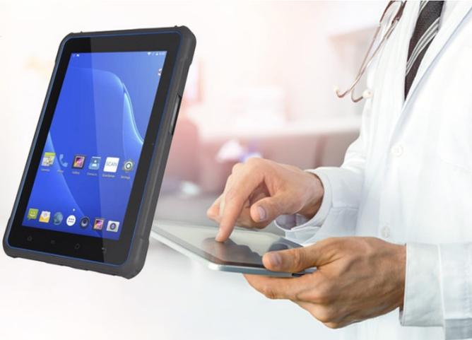
The BCX-801UHF has been designed to be a 'go anywhere' work companion. It has an 8" colour touchscreen which is large enough to display sharp, detailed imagery, yet compact enough to fit neatly into a bag/satchel.
